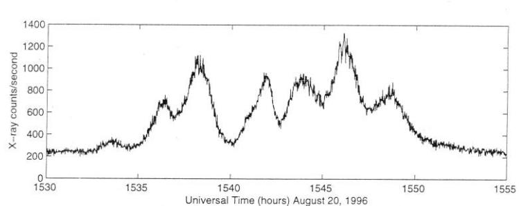
Figure 1. X-ray imager data taken during the relativistic electron precipitation event of August 20, 1996. The X-ray count rate between 20 and 120 keV is averaged over 1 s. The 10–20 s modulation is most clearly visible superposed on the peak starting near 1545 UT.
