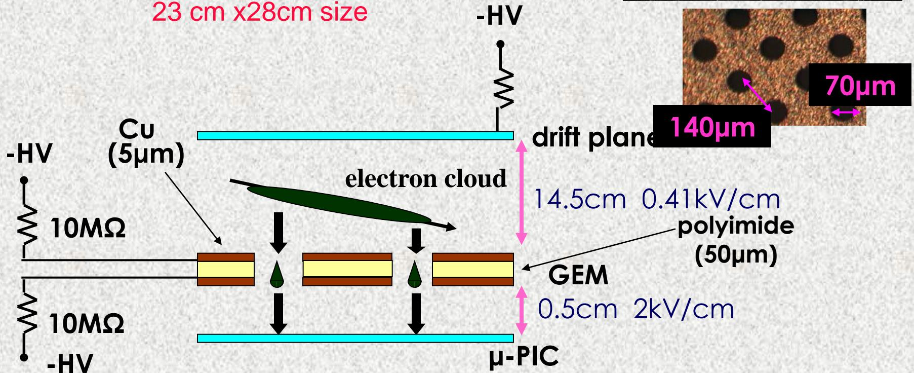
Electrons (~2 in one pixel) bare amplified by the GEM and the  $\mu$ -PIC with a gain of  $>2 \times 10^4$
