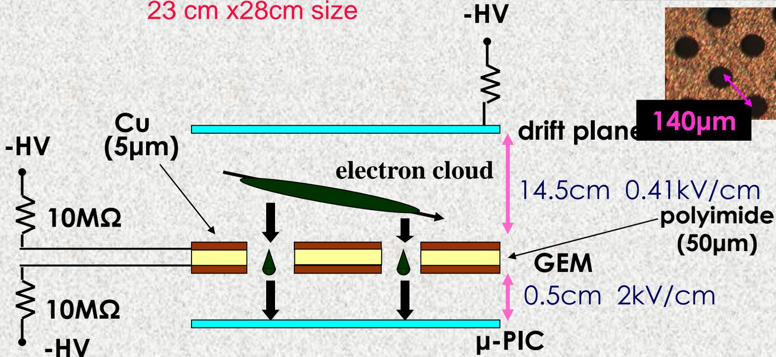
Electrons (  $\sim 2$  in one pixel) are amplified by the GEM and the  $\mu$ -PIC with a gain of  $> 2 \times 10^4$
