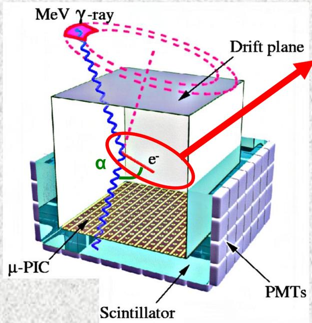
1. Determination of the direction of each gamma ray
